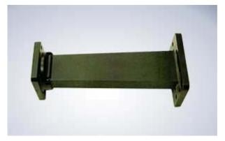
1.70 - 22.00 GHz Performance Frequency 1.25 Typical Max VSWR (VSWR varies with design) Numerous Flange Configurations available Aluminum (6061) or Brass WR Waveguide Available
